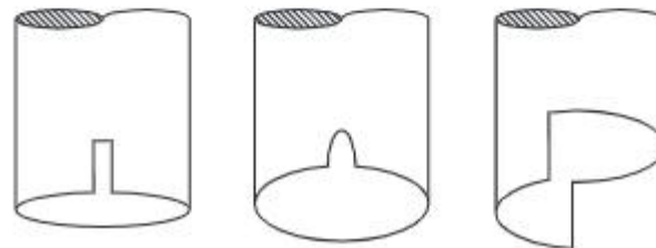
(b) Different shapes of the dip pipe (or bubbler tube)
